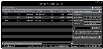
3 Modify the IP address. The default IP address of this camera is 192.168.226.201. Click the information of the camera listed in the above table to show the network information on the right hand.
